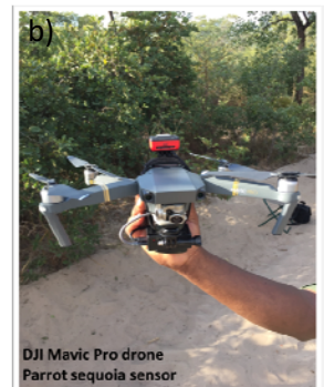
a) Field sampling protocol for nine validation sites and the b) DJI Mavic Platform and Parrot Sequoia sensor flown for data collection.
